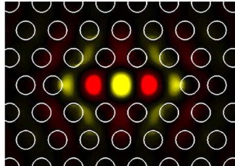
Fig. 2: Electric field profile of the L3 cavity mode.
