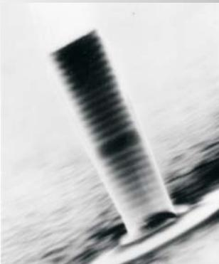
Scanning electron micrograph of a micropillar.
