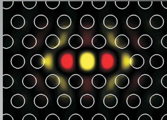
Field profile of an optical mode in a photonic crystal cavity.
